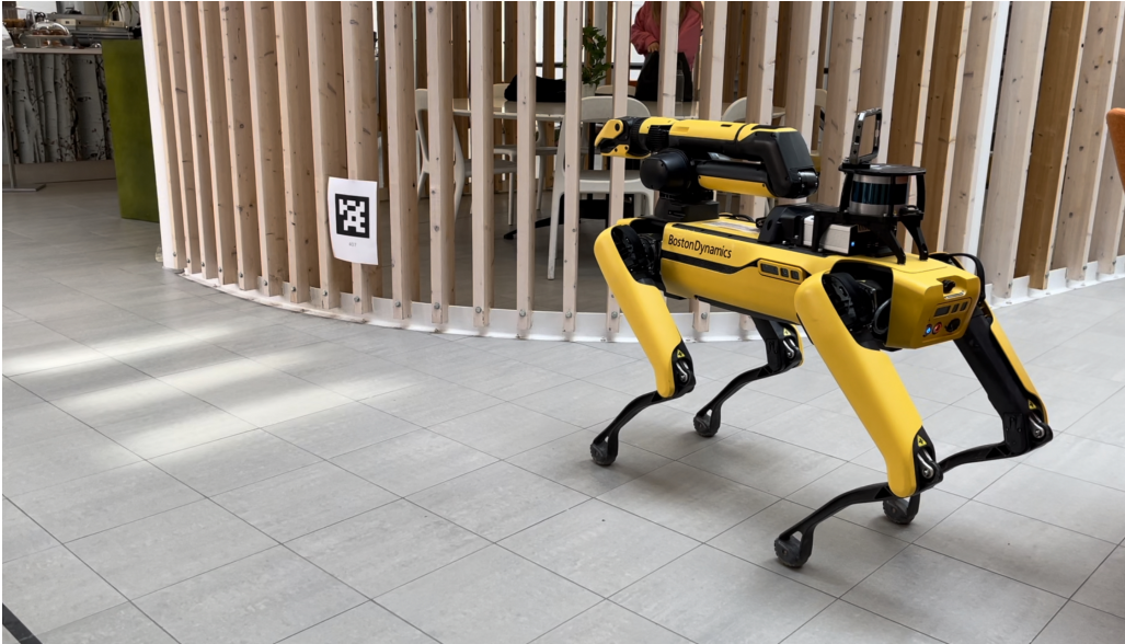
Figure 6.2: AprilTag fiducial near Spot during indoor localization test
