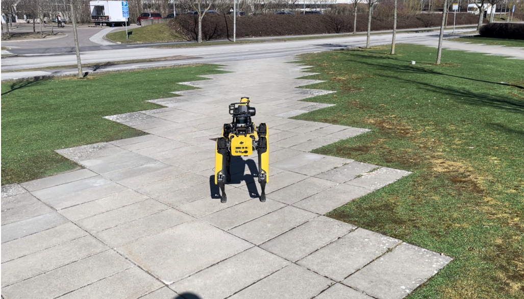
Figure 6.5: Spot robot during localization test in a park
